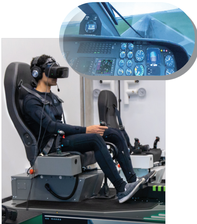
Aerospace engineering graduate student Michael Morcos tries out one of the BRUNNER motion-base VR simulators installed at University of Maryland (UMD) assistant professor Umberto Saetti's Extended Reality Flight Simulation and Control Lab. UMD is one of the only universities in the U.S. to house motion-base VR simulation equipment, which can reproduce flying conditions in a wide variety of aircraft.
